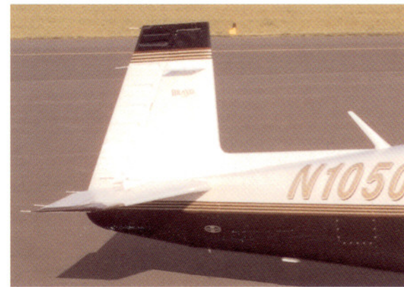
The signature Mooney all-trimming tail reduces drag to squeeze maximum performance out of every drop of fuel.
