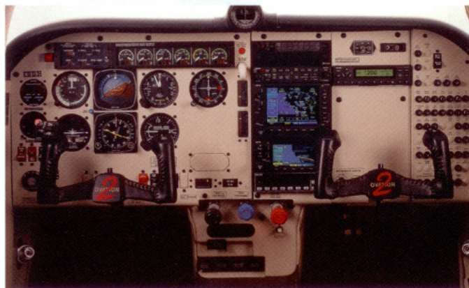
A complete GARMIN avionics stack plus the premium Bendix King KFC 225 autopilot/flight director is standard.
