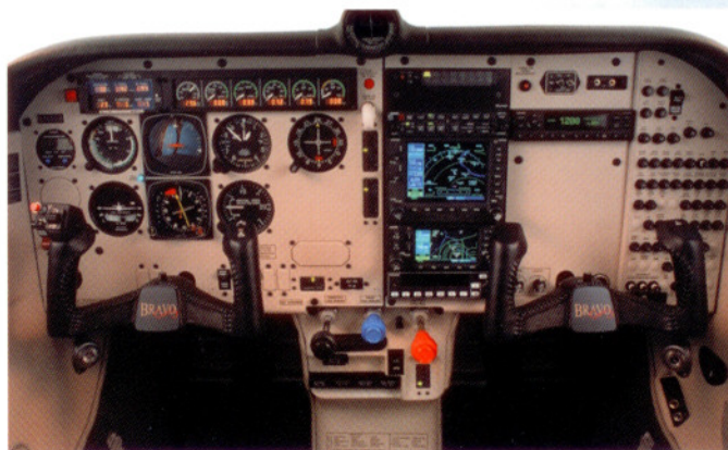
Fully IFR equipped panel backed by dual batteries, dual alternators and a standby vacuum pump as standard equipment.
